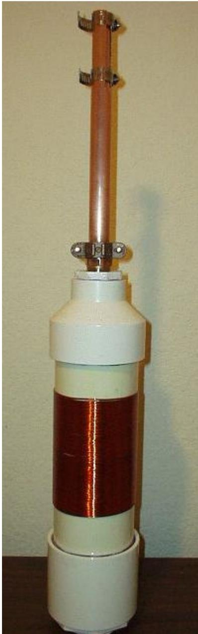
When mounting the completed antenna onto the mast, it should be obvious that the 1 1/2" steel mast screws into the bottom of the coil form.
